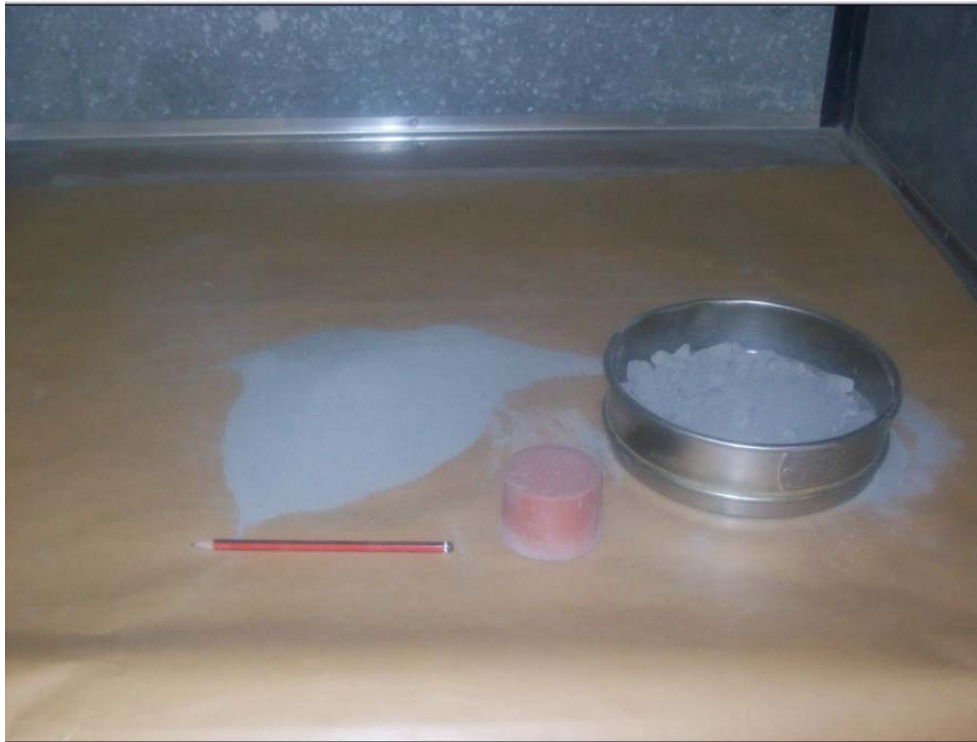
Figure 4.3: Screening of sample using 850 µm sieve and a rubber bar.
