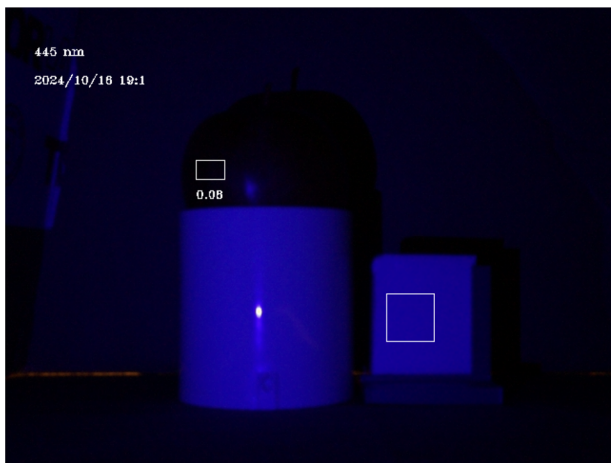
Fig. 4. An LED with center wavelength at 445 nm illuminates an apple and a Teflon reference. At 445 nm, the apple reflectance is very low and is barely visible in the image.
