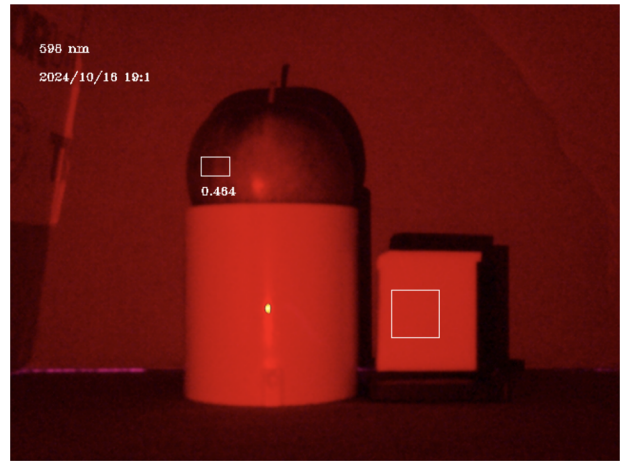
Fig. 5. An LED with center wavelength at 596 nm illuminates an apple and a Teflon reference. At this wavelength, the apple reflectance is about 50%.
