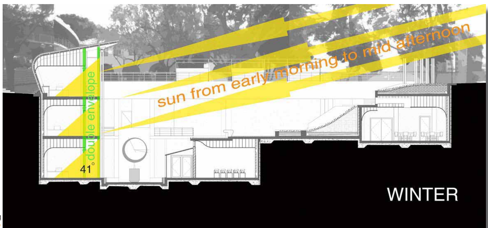
Winter incidents and heating Fig.129
