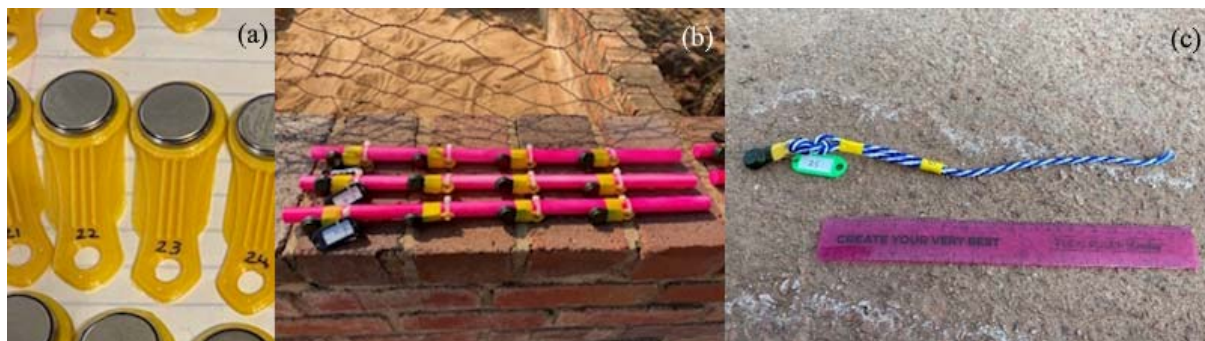
Figure A2. Images of (a) the 3D printer holders, (b) dowel iButtons, and (c) single iButtons.
