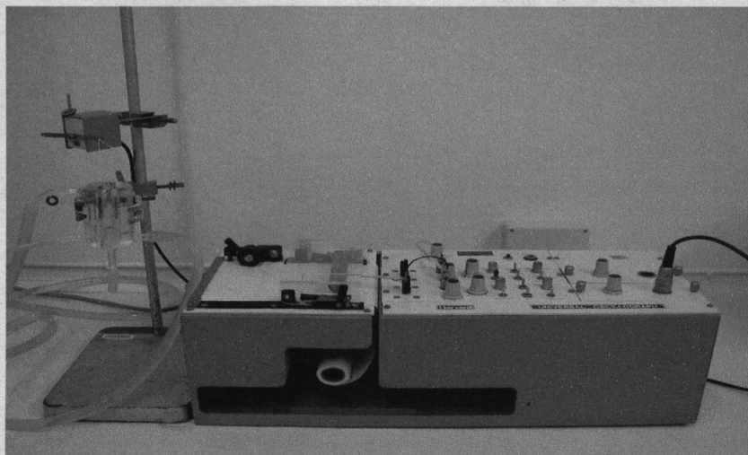
Fig 2: Experimental bath, Harvard isotonic force transducer and recorder.
