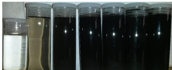
Figure 3.1: Carbon black nanofluids from left: 0.00; 0.0005; 0.001; 0.003, 0.005, 0.01, 0.05 volume % carbon black.
