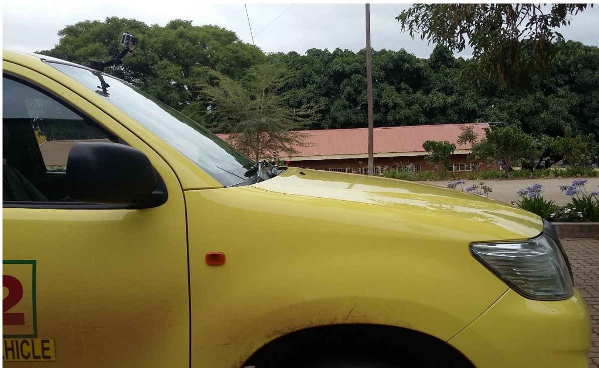
Figure 3-3: Setup of GoPro Hero 6 on Toyota Hilux construction vehicle
