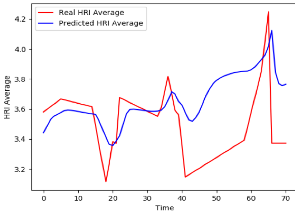
Figure 3-22: Predicted and Real HRI vs time for ts = 70 , epochs = 100, neurons = 50 and batch size = 5
