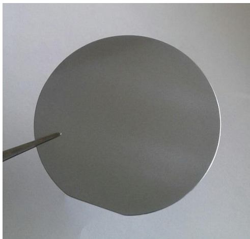
Figure 2-1: A picture showing a 3 inch Czochralski-grown Si wafer used in this study.
