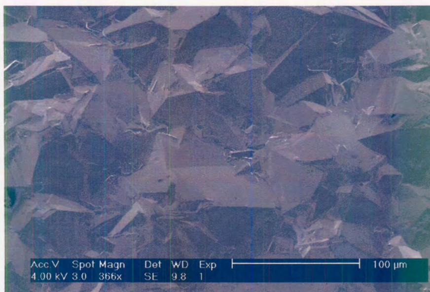
Figure 5.8 : SEM image of the as-received CVDBD4(2) sample
