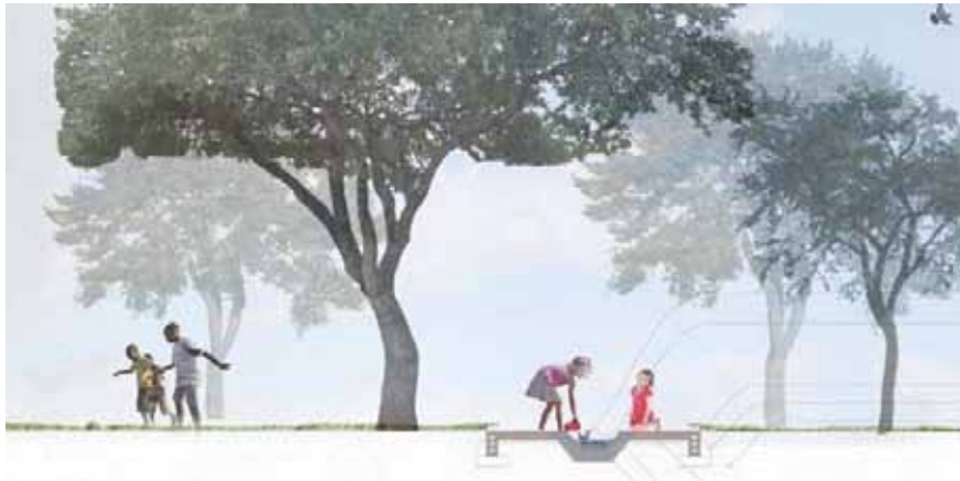
Figure 26 A section indicating the open concrete channel with a typical weir where children might play (illustration: Rossi, 2012).
