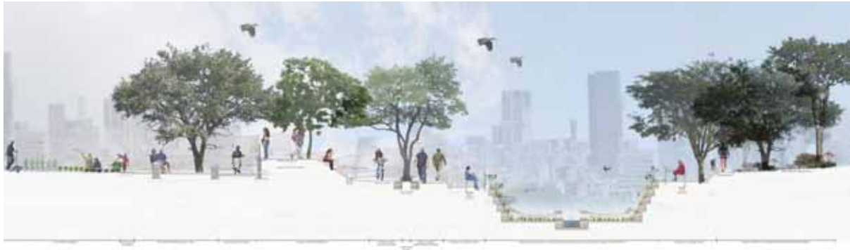
Figure 24 Section indicating one of the raised platforms, the pedestrian and cyclist pathways, and the de-channelized Walker Spruit alongside the proposed urban forest (Illustration: Rossi, 2012).
