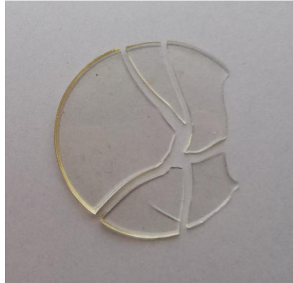
Figure 25: Sample D of Set 06, one thin layer of Paraloid™ B-72 in the room temperature silicone mould. Photograph by author.
