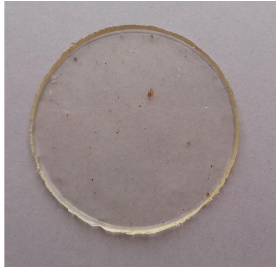
Figure 33: Sample B of Set 10, multiple thin layers of the hybrid mix. Photograph by author.
