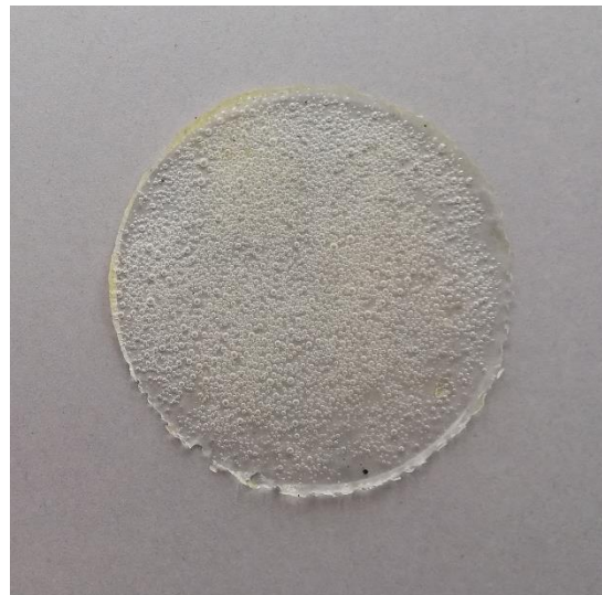
Figure 27: Sample B in Set 07, multiple thin layers of Paraloid™ B-48N. Photograph by author.
