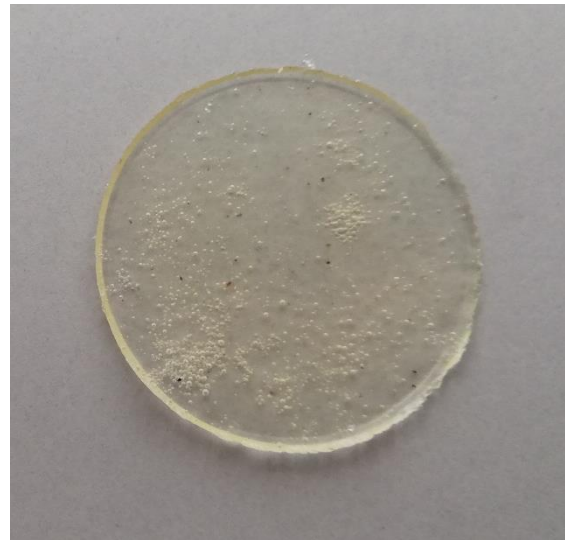
Figure 29: Sample B of Set 08, multiple thick layers of the hybrid mix. Photograph by author.
