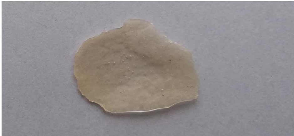
Figure 18: A sample of thermocasted Paraloid™ B-72 made within a baking parchment vessel. Photograph by author.
