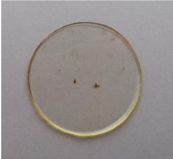
Figure 22: Sample A of Set 06, one thick layer of Paraloid™ B-72 in the preheated silicone mould. Photograph by author.
