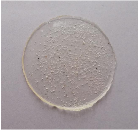
Figure 32: Sample A of Set 10, one thick layer of the hybrid mix. Photograph by author.
