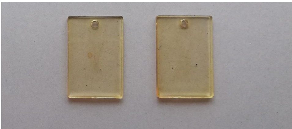
Figure 19: Set 04 of samples using the thermocasting technique at 80°C. Photograph by author.
