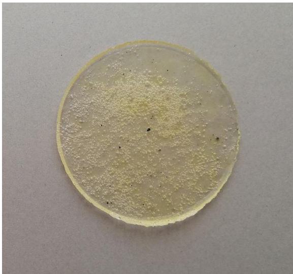
Figure 26: Sample A in Set 07, one thick layer of Paraloid™ B-48N. Photograph by author.
