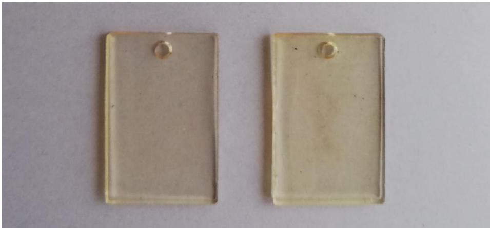
Figure 16: Samples from Set 02 of thermocasting Paraloid™ B-72. Photograph by author.
