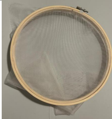
Figure 6: 500-micron nylon mesh from Dawning Filters in embroidery hoop. Photograph by author.
