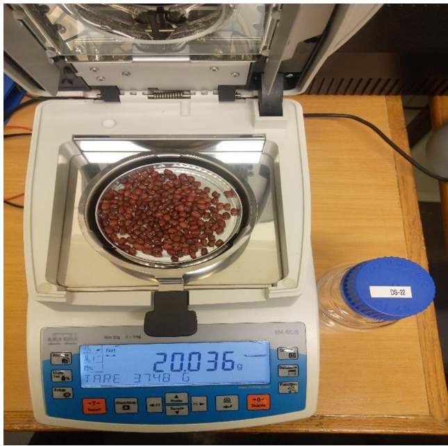
FIGURE 1 Measuring of studied cowpea sample with moisture content analyzer.
