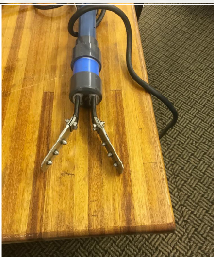
Figure 3: Electrode prongs of the e-stunner wand with three metal buttons on each electrode to improve skin contact and electrical conductivity.
