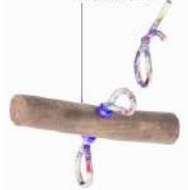
DETAIL 2 ROPE JOINT
