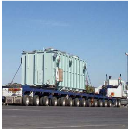
Figure 7: A transformer being transported via truck
