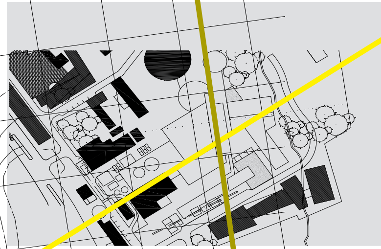
Fig. 6.14_ the use if grids on site
