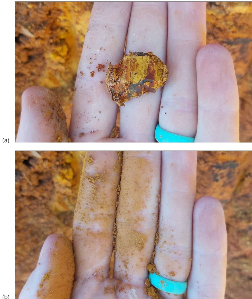
Figure 8-2 (a) Sample 2835 with structure intact (b) Sample 2835 after smeared with light finger pressure (photographs taken by D Swart)
