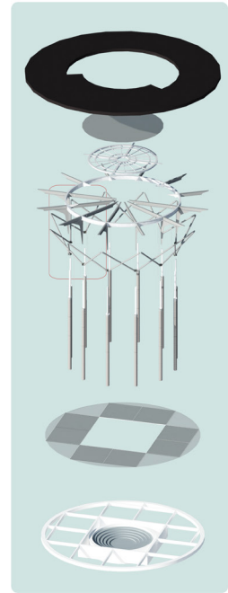
Exploded structure of the central space
