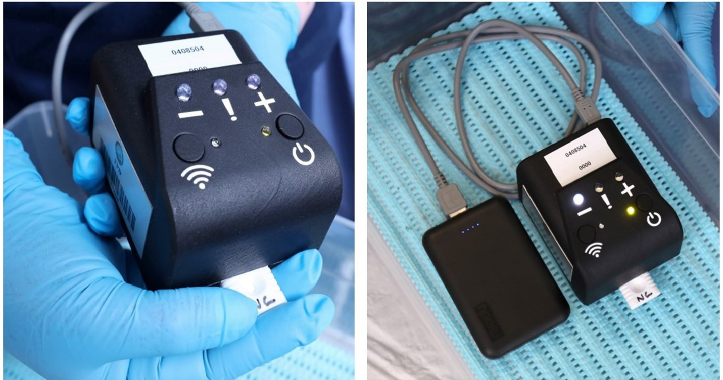
Fig 3. NG-LFA reader and portable power bank. Implementing staff followed each step for testing set-up through the guidance of an instruction leaflet (S1 File).
