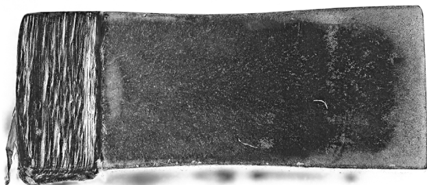
Fig. 11. Micrographs of fracture surfaces of the OCC/1.8CB/0.25S specimen.
