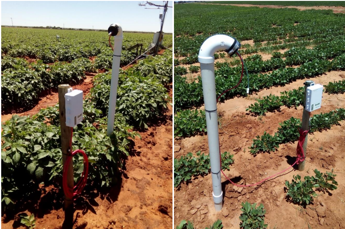
Appendix 3: Decagon G3 drainage lysimeter access pipe and EM500 data-logger in potato (Left) and subsequent groundnut (Right).
