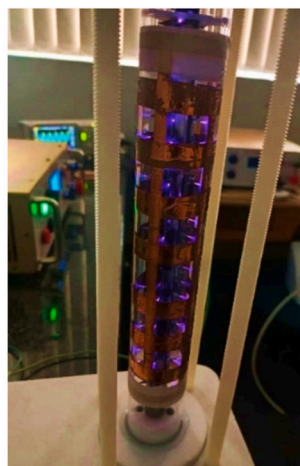
Fig. 1. Experimental arrangement for the tramadol degradation process (a) schematic illustration of the setup (b) DBD plasma reactor showing purple streamer discharges at the edges of the multi-pin electrode.
