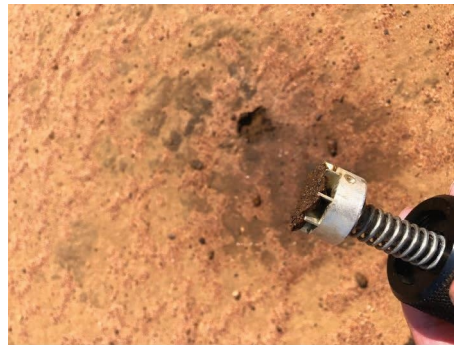
FIGURE 13: Jagged edge hole with scattered pieces of surface crust at crust strength measurement in a control plot.
