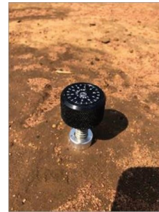
FIGURE 5: The Humboldt H-4212MH pocket shear vane tester (small vanes).
