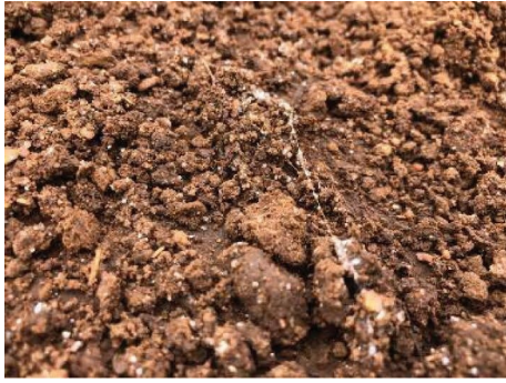
FIGURE 10: Structure formation and stabilisation effect of PAM.
