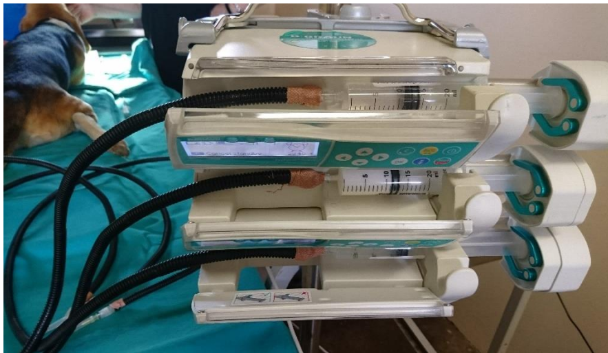
Figure 1: Electronic syringe driver systems used to administer the anaesthetic induction drugs. Note the black general purpose electrical trunking material used to cover each extension set to obscure visibility.
