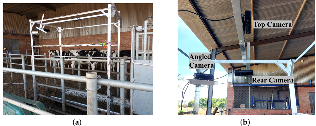
Figure 2. Data collection frame setup: (a) Placement of data collection frame over crush; and (b) Camera placement on frame.
