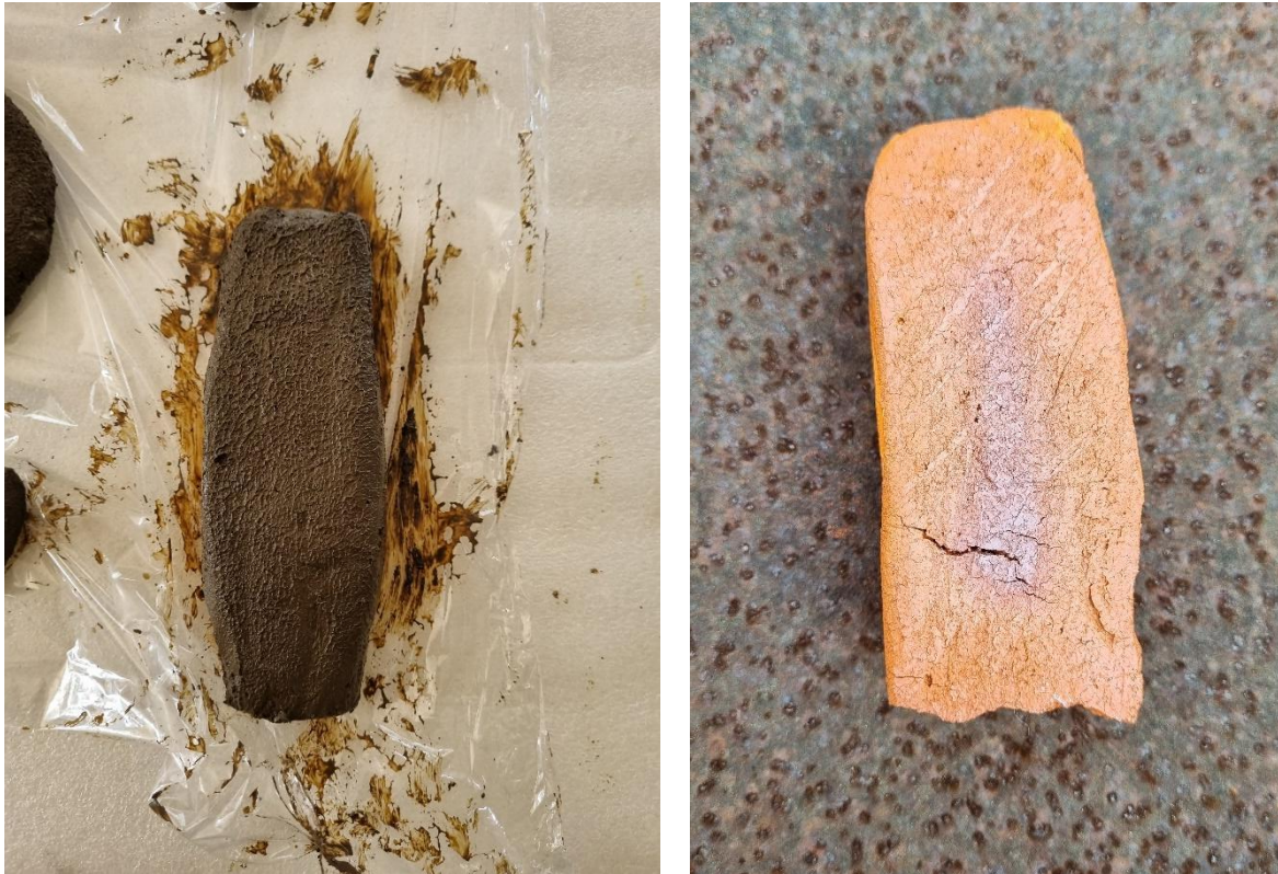
Figure 53: (left) the log-shaped form prior to firing; and (right) post-firing (photo credit: Chelsea Roberts, 2023).
