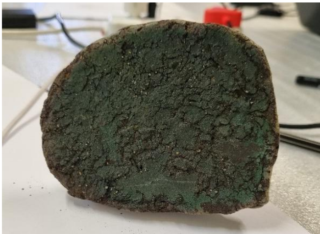
Figure 29: This is an image showing the base of the leopard ashtrays with the crumbling blue/green layer (photo credits: Chelsea Roberts, 2023).
