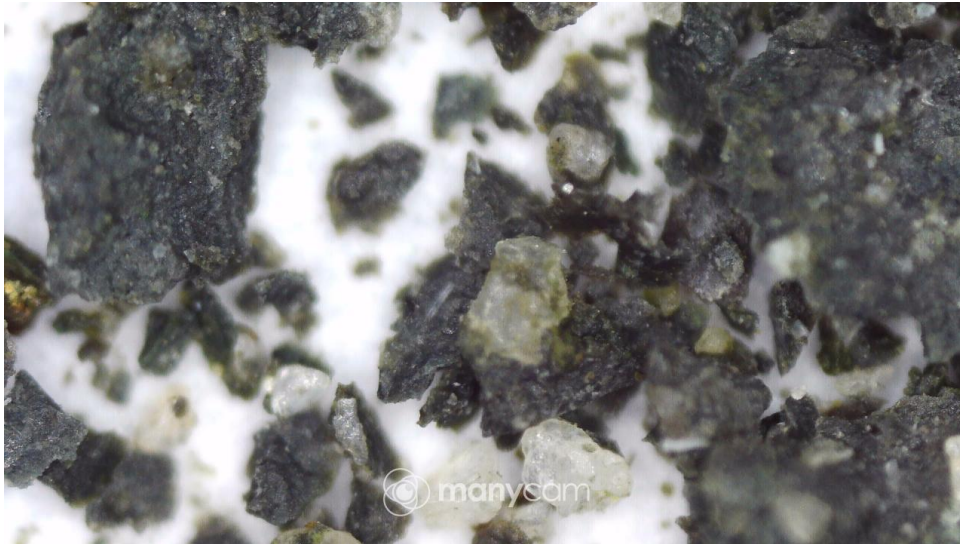
Figure 33: An image at 100x magnification showing the composition of the crumbling material, specifically focusing on the unknown green colouration (photo credits: Chelsea Roberts, 2023).
