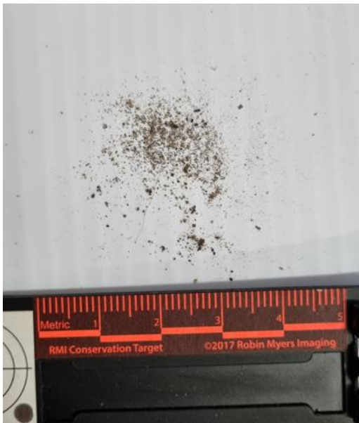
Figure 12: Powdering material that is currently coming off the Bushman sculpture (photo credit: Chelsea Roberts, 2023).
