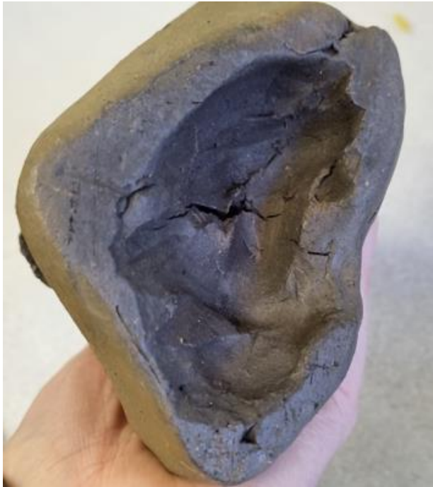
Figure 24: The base of the sculpture reveals the drying cracks present in the sculpture (photo credits: Chelsea Roberts, 2023).
