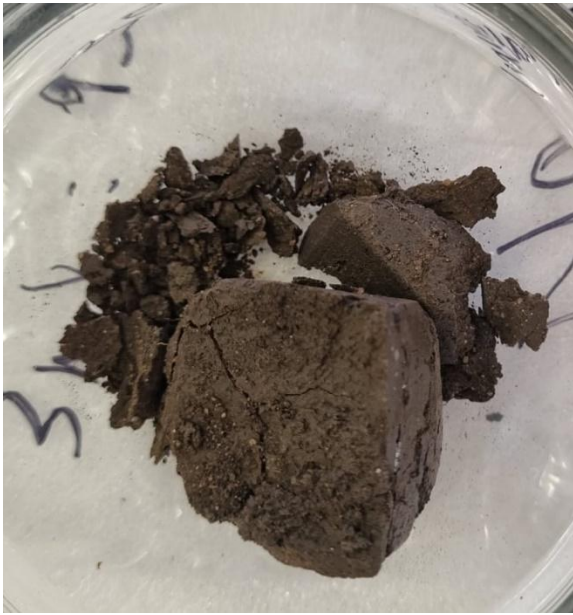
Figure 44: Clay cube after capillary consolidation with 7% Raviflex in Ethanol (Photo Credit: Chelsea Roberts)
