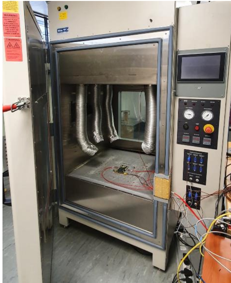
Figure 3.5. HALT chamber at Hensoldt GEW Technologies.
