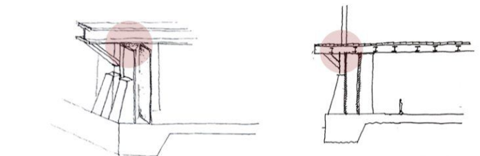
SKETCH SECTION THROUGH AUDITORIUM 3DCP WALL
