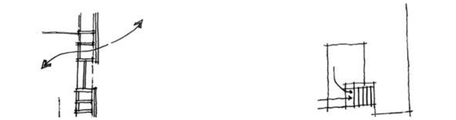
choice of white corrugated steel and clear corrugated polycarbonate as cladding materials, Permeable facade on shaded edge
