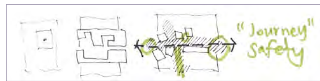
Figure 22. In the process of refining the safety concept, multiple iterations were undertaken to meticulously craft building forms that would best serve the overarching goal. The primary aim is to create an environment where safety is paramount, offering users a clear and easily navigable path. This involves designing spaces with unobstructed sightlines, allowing individuals to see through the area and have a comprehensive understanding of their surroundings as they traverse the space. Every aspect, including building edges, overhead planes, and interstitial spaces, undergoes careful consideration to prevent any elements that might contribute to a sense of alienation for users as they move through the project. This thorough approach ensures that the safety concept is not only a theoretical consideration but a tangible and integral part of the project's design.
