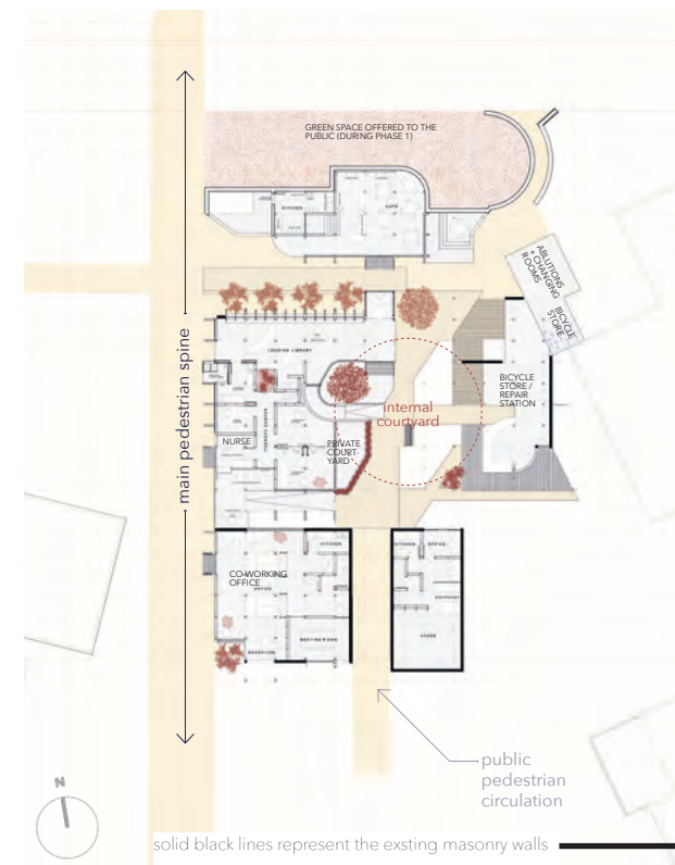
Figure 41. Revised ground floor plan - specific focus was given to the pedestrian circulation within the interventions.
