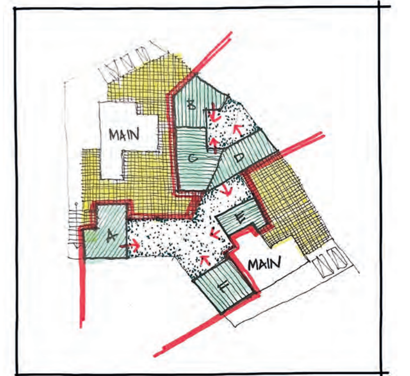
Sketch exploring the options for densifying the interstitial spaces between the residential homes.
