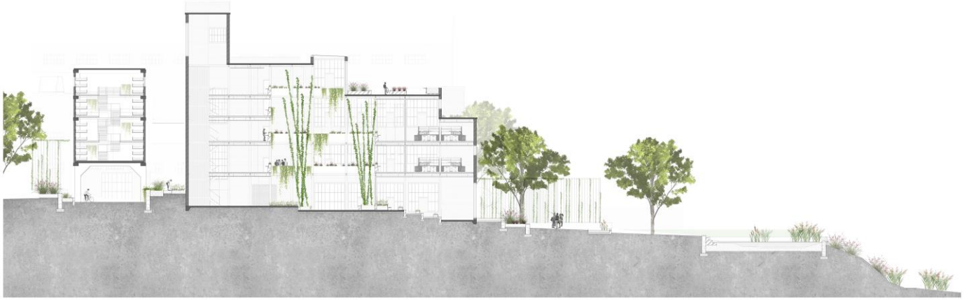
Figure 31: Section A through the existing building connecting to the surrounding public landscape and Phytoremediation research spaces (incomplete). The greyed out walls/floors demonstrate the existing structure.
