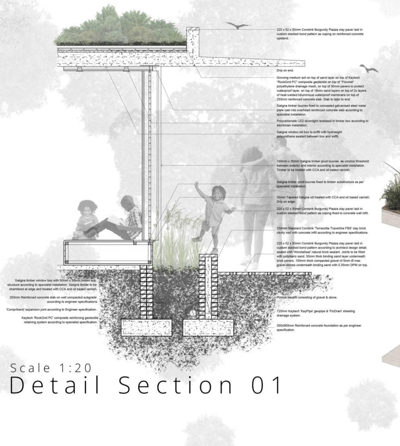
1. 220 x 52 x 50mm Corobrik Burgundy Piazza clay paver laid in custom stacked bond pattern according to architect design detail, sealed with 'WondaSeal' natural brick sealant. Joints to be filled with polymeric sand. 50mm thick binding sand layer underneath brick pavers. 100mm thick compacted gravel of 5mm Ø max gravel stones underneath binding sand with 0.35mm DPM on top of 85mm reinforced concrete slab.
