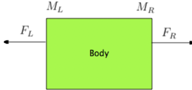
Figure 6.2: Direction of force and moment on the body
