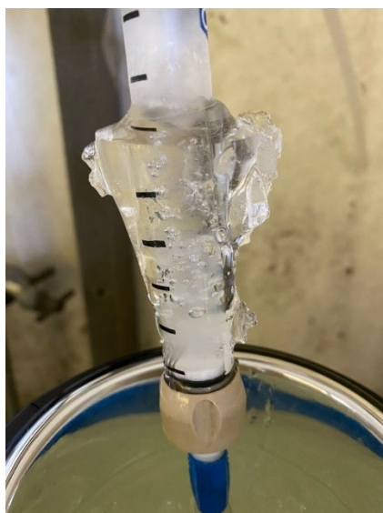
Figure S-10: Reaction mixture “freezing” below -30\text{ }^{\circ}\text{C}
