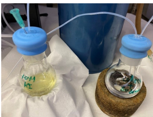
Figure S-6: 10 mL of 1.0 M KI solution reaction with 0.25M substrate (alpha-methylstyrene) present
