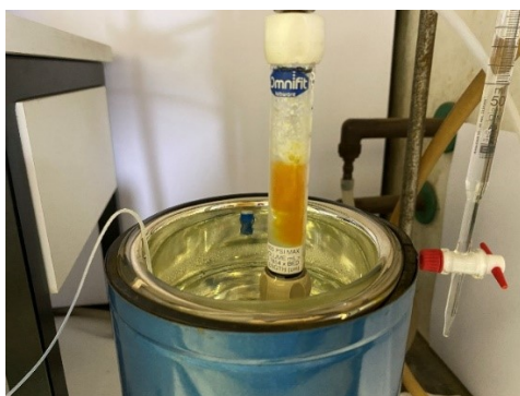
Figure S-8: Pumping 10 % KI solution in Methanol through the reactor
