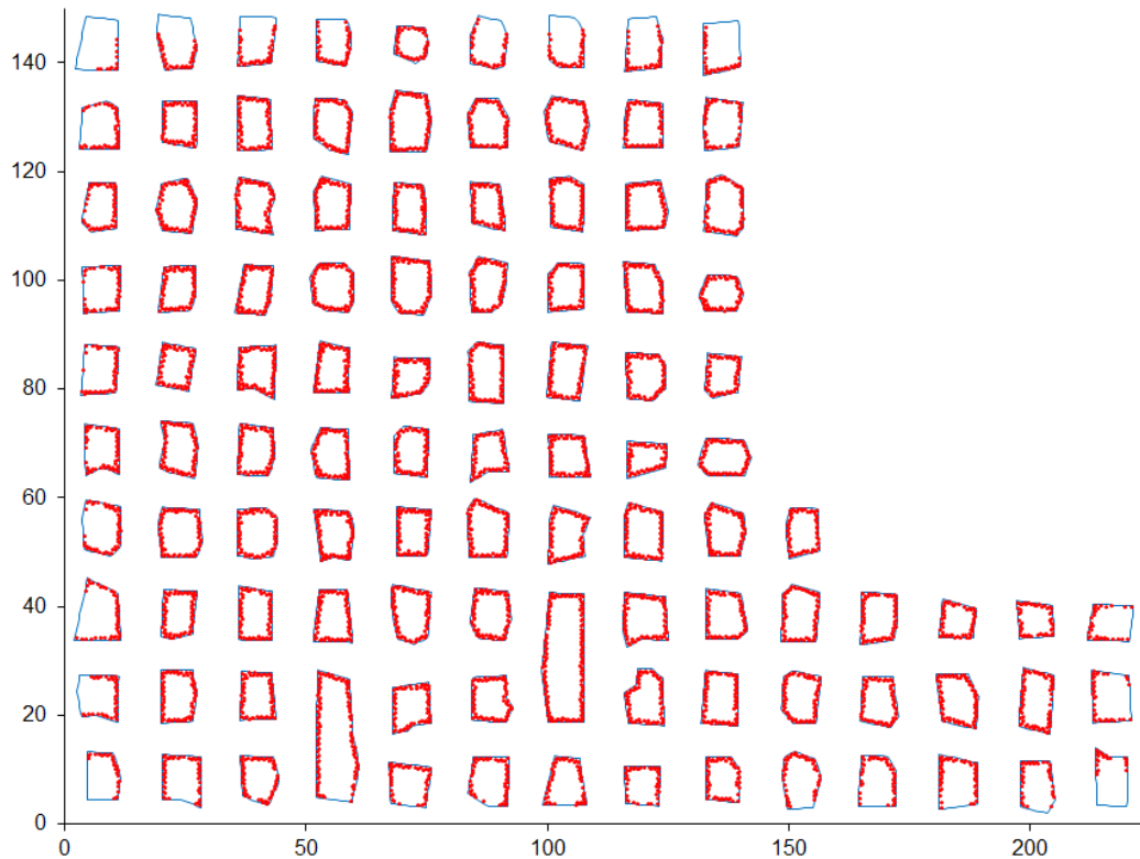
Figure 5-7. Predicted pillar spalling at 600 m below surface.
