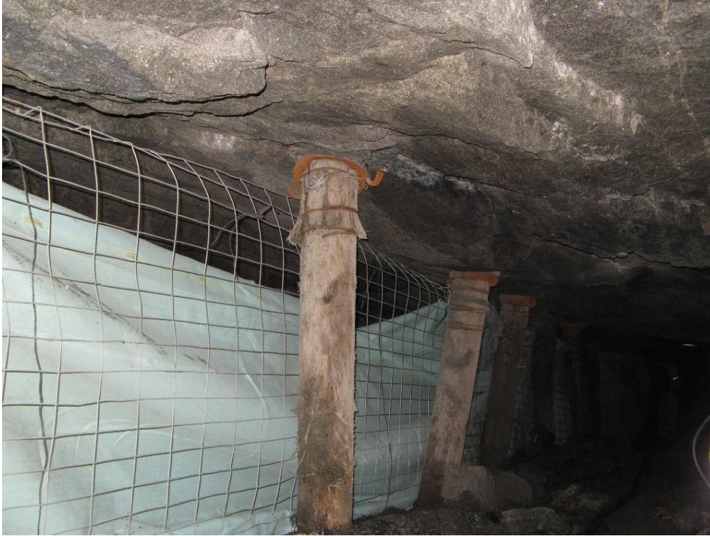
Figure 2-22. A backfill paddock before it is filled with backfill (courtesy of D. F. Malan).
