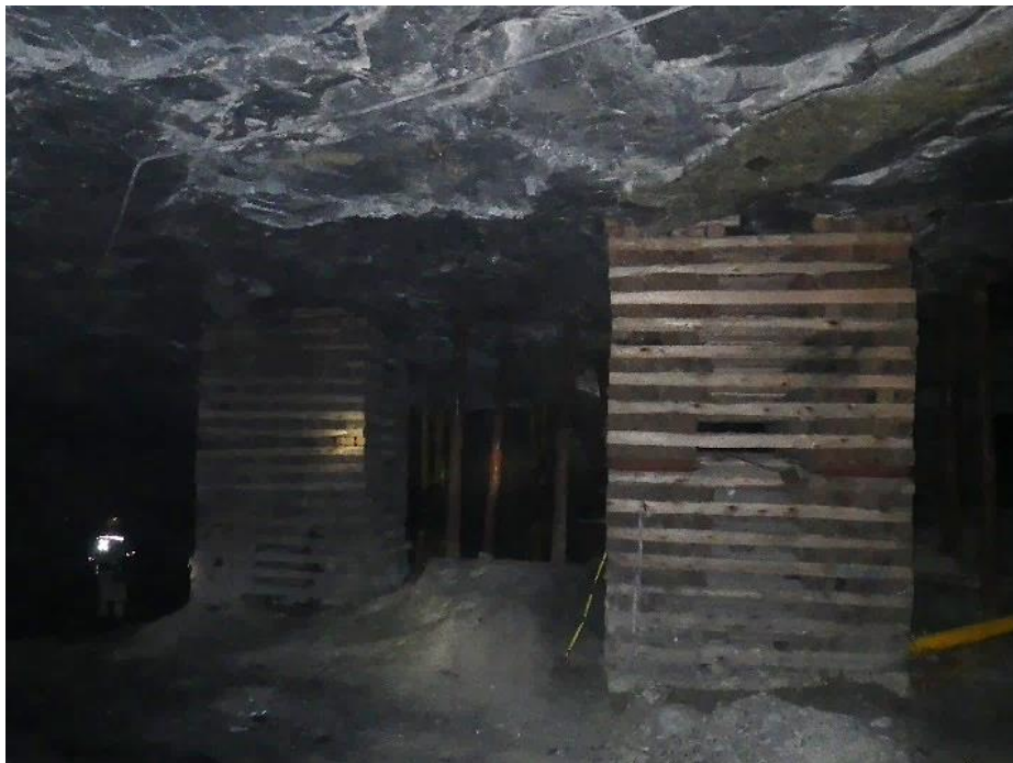
Figure 2-43. Castle packs in the area where pillar extraction is occurring (D. F. Malan 2023, pers. comm.).
