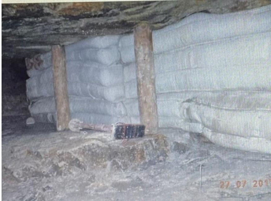
Figure 2-46. Grout packs used at Modder East for pillar extraction (D. F. Malan 2023, pers. comm.).
