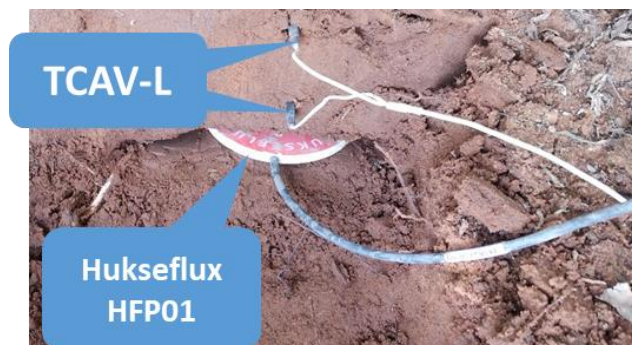
Figure 3.110 A Hukseflux HFP01 soil heat flux plate in parallel with two TCAV-L soil temperature averaging probes.
