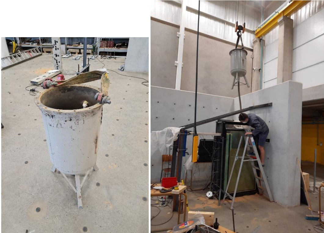
Figure 3-12: Hopper used to pluviat sand into the steel box.
