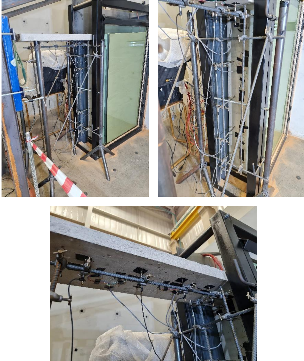
Figure 3-11: LVDT frame used for connecting all LVDTs (abutment wall and deck portion).
