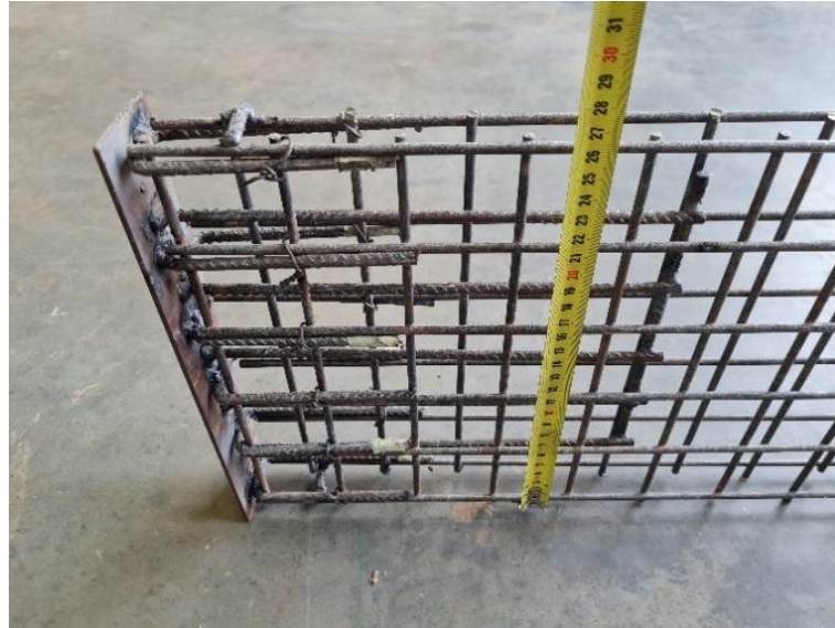
Figure 3-6: Deck end connection for the abutment specimens.
