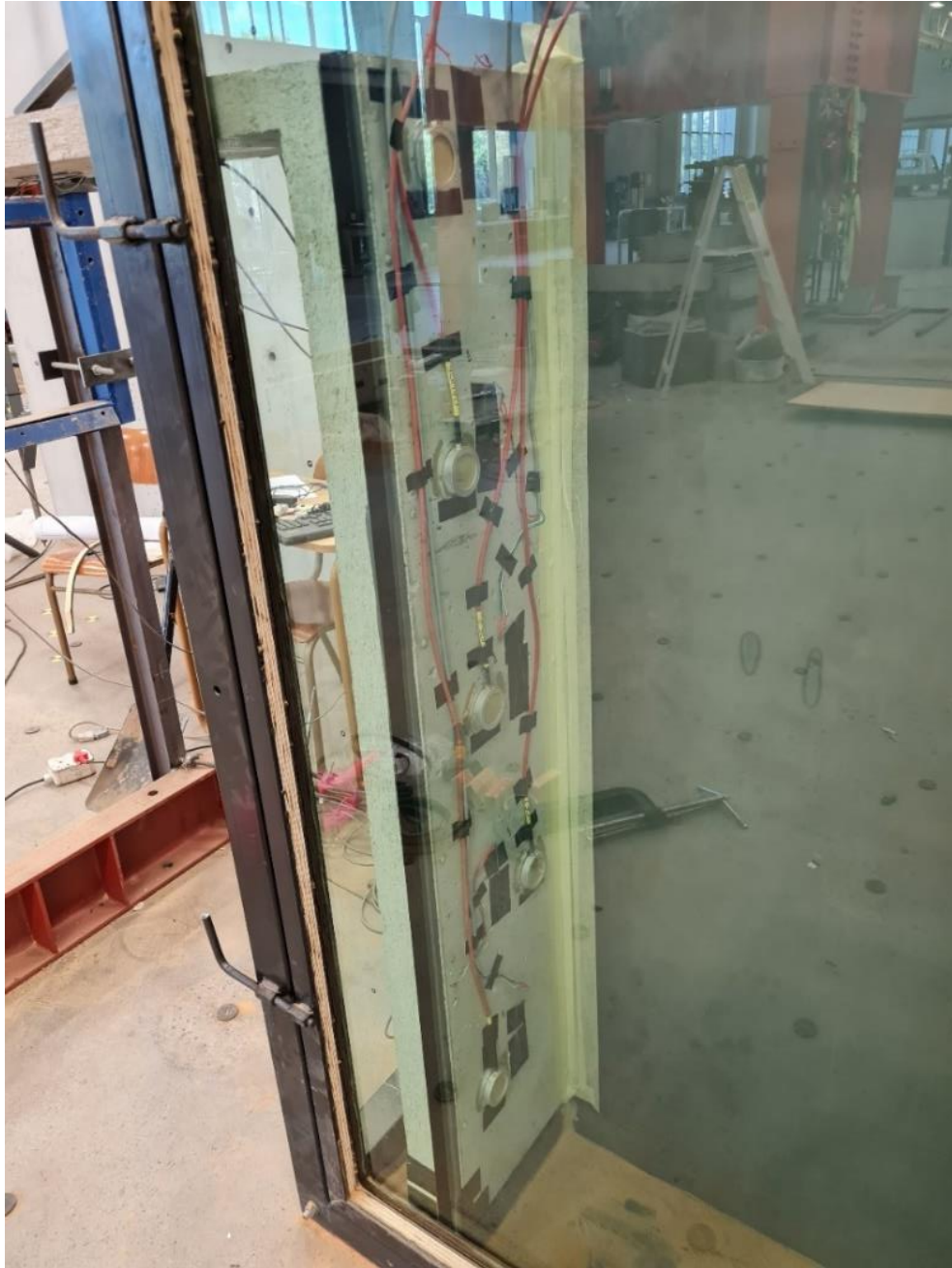
Figure 3-13: Sealing strips used for concrete-glass interface and masking tape used for the concrete-steel sheeting interface.
