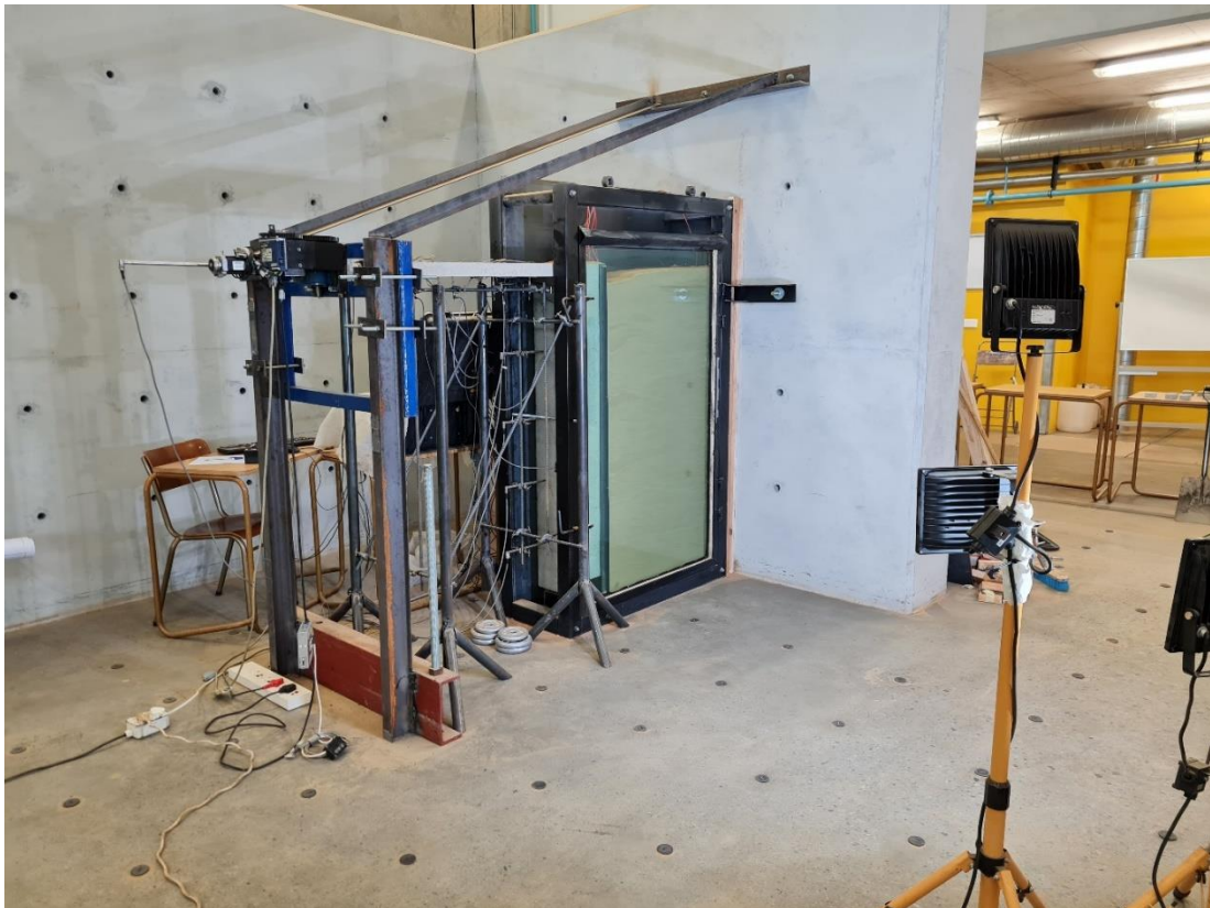
Figure 3-1: Complete test setup for an abutment-deck specimen.
