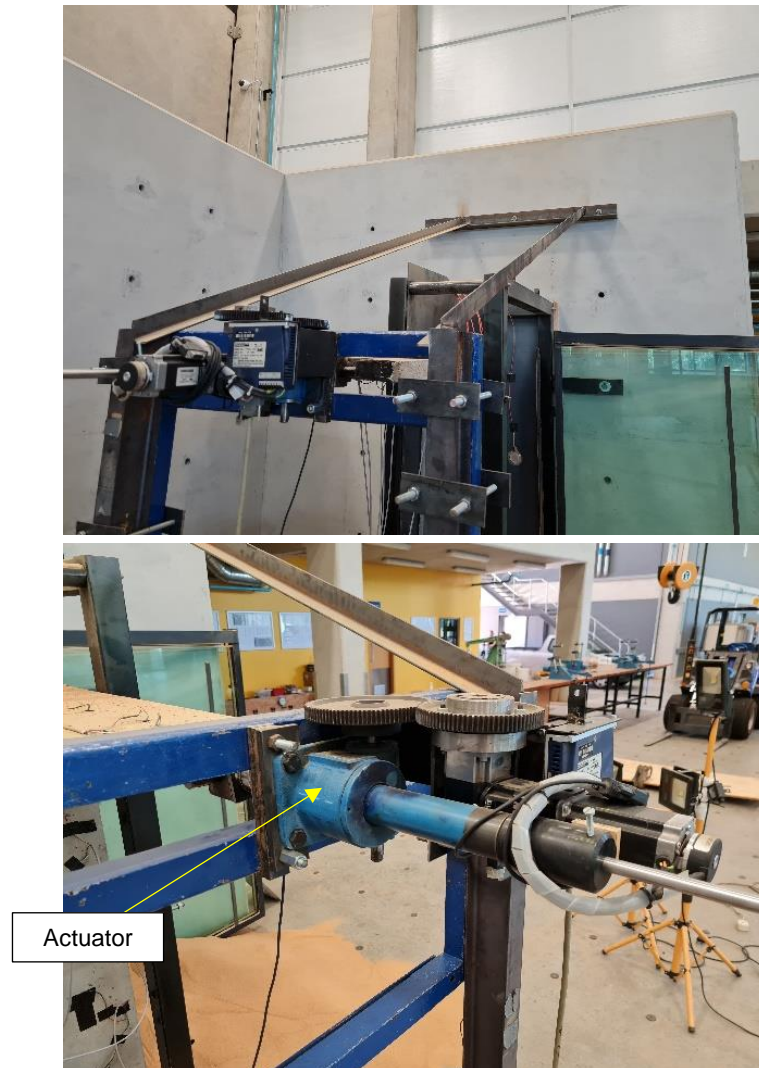
Figure 3-14: Actuator positioned onto mounting frame.
