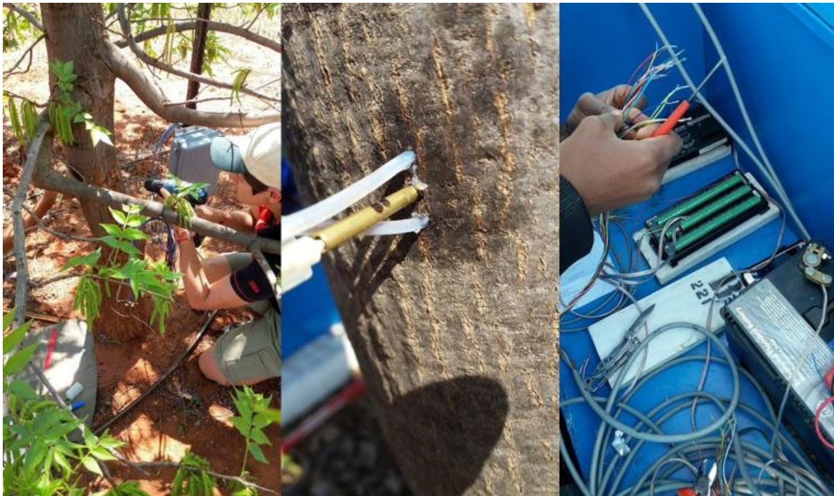
Figure 3.5 Installation of the sap flow equipment on the experimental farm.
