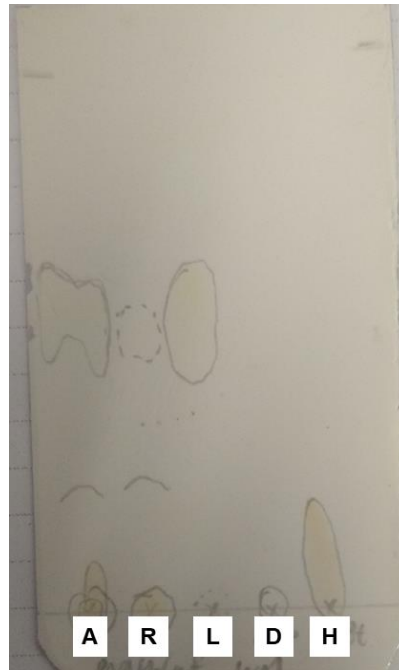
Figure 2.23: TLC of Lumf conjugation reaction to PNAM. A – All materials; R – chemical reaction of Lumf conjugation to PNAM; L – lumefantrine; D – dimethylaminopyridine (DMAP); H – hydroxybenzotriazole (HoBT). TLC was run using a solvent system of ethyl acetate: hexane at a ratio of 4:1.
