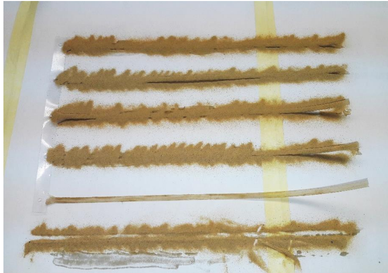
Figure 3-20. Surface preparation of the reinforcement strips.
