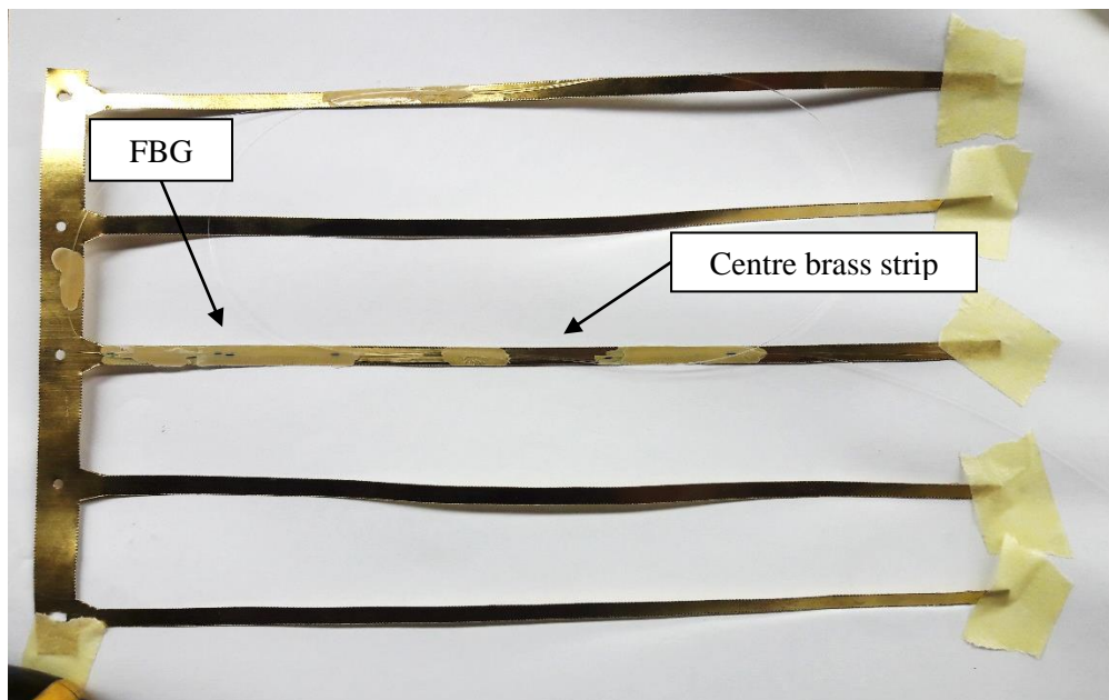
Figure 3-13. FBGs glued onto the centre brass reinforcement strip.
