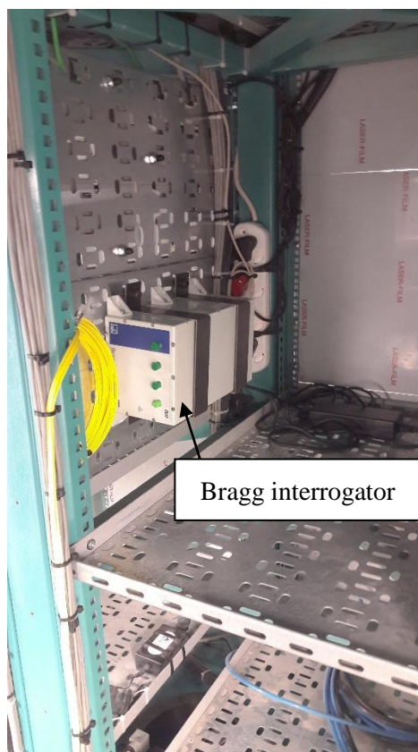
Figure 3-14. HBM fibre Bragg interrogator in the centrifuge.
