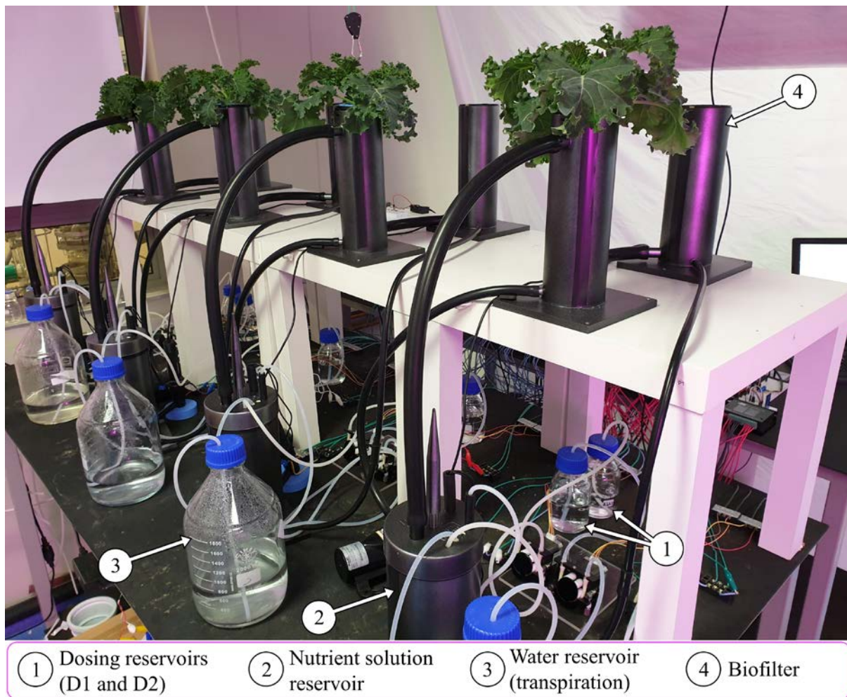
Fig. 5: Annotated photo of the experimental setup showing four independent hydroponic systems. In each experiment, all four systems were operated in parallel under the same conditions (thus yielding four repeats). Each system is labelled “system 1” to “system 4” (from right to left) in the subsequent data reports.
