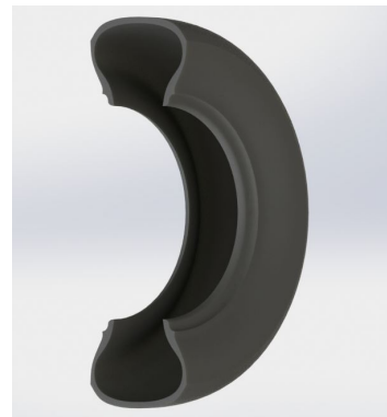
(b) TM700 CAD cross-section with the tread lugs shaven off
