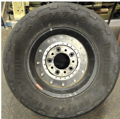
(a) A Trelleborg TM700 with the tread lugs removed
