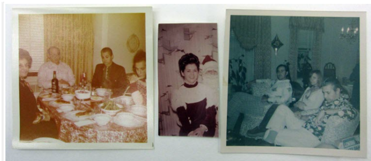
Figure 28. - Colour fading of chromogenic photographs, here each photograph is fading in a different colour spectrum. The first is yellowing, the second is turning magenta and the third is turning blue (Government of Canada, Canadian Conservation Institute. CCI 129982-0019).
