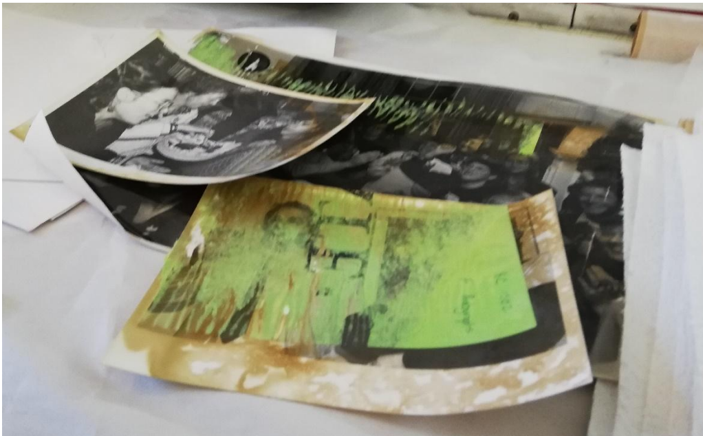
Figure 31 - Water damage as a consequence of firefighting efforts, photographs have stuck together and dirt and soiling solubilised in the water has now soiled and stained the photographs. Photograph courtesy of Isabelle McGinn UCT, Jagger reading room fire salvage 2021.
