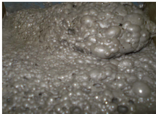
Fig. 1. PCB CF froth in the flotation cell under natural hydrophobic response.
