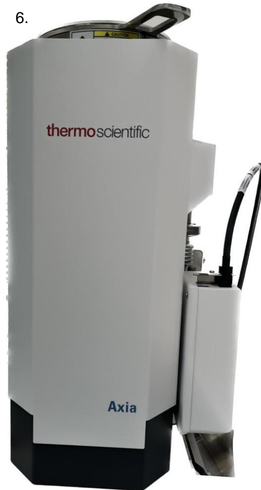
Figure 6: Scanning electron microscope used to record images of zirconia specimens and diamond burs (Axia ChemiSEM, Thermo Fisher Scientific Inc., USA).
