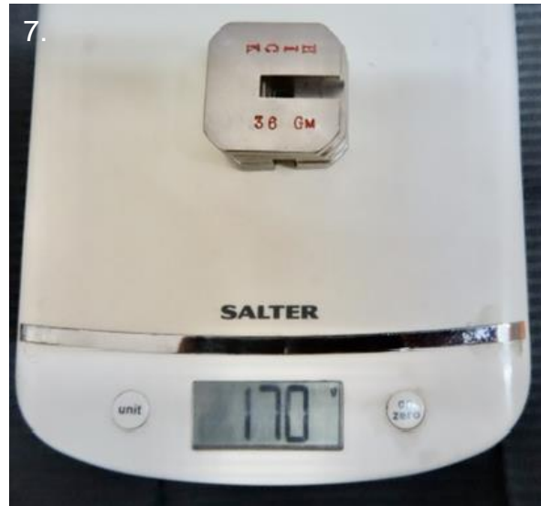
Figure 7: Salter Digital Scale used to measure 170g weight.
