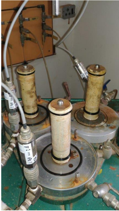
Figure 22: The 4-layer Diamond mesh reinforced triaxial test set up.
