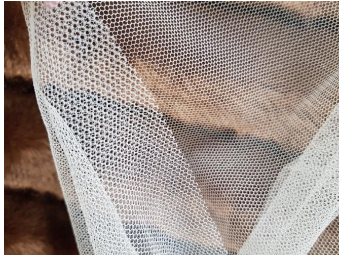
Figure 15: Image showing the Mosquito Net (fabric) reinforcement
