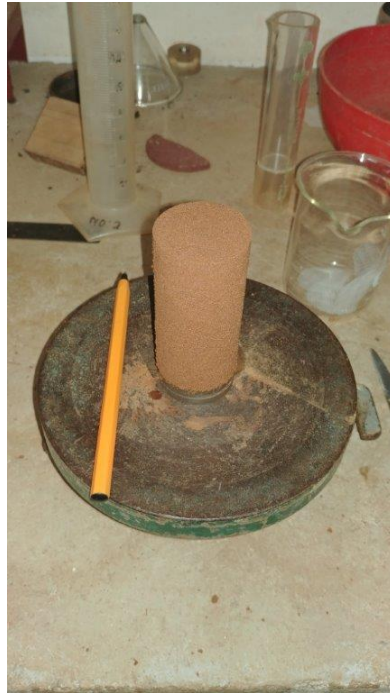
1162 Figure 18: Test set up of the unreinforced sample.
