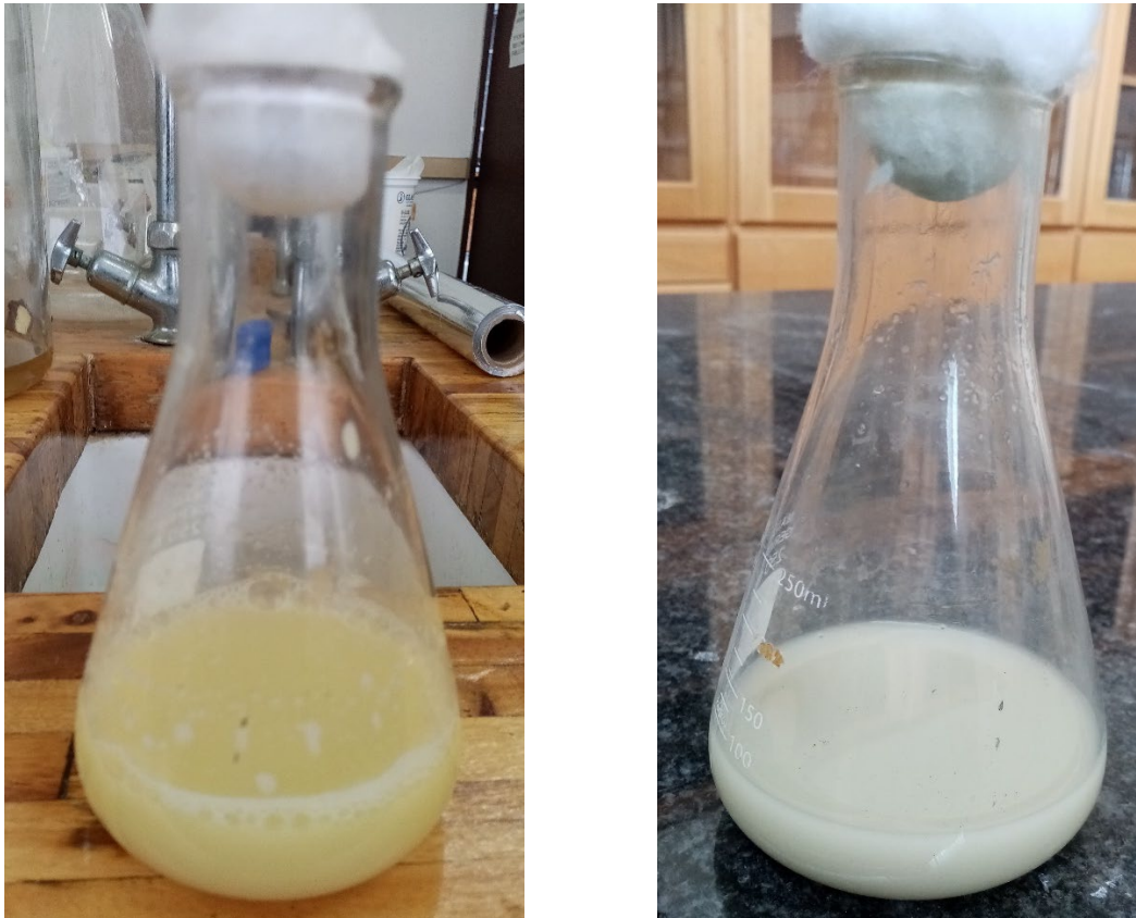
Figure 3-1: Erlenmeyer flask for Cr(VI) reduction experiment (a) 100 mg/L Cr(VI) before incubation (b) after 24 hours of incubation
