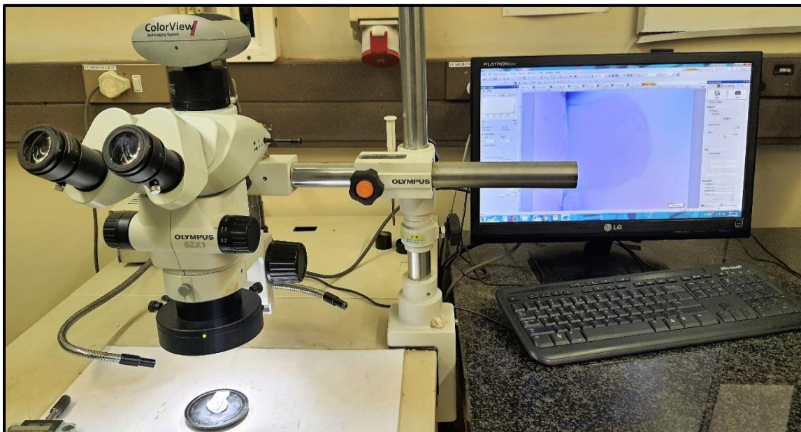
Figure 3-28: Olympus SZX7 Stereomicroscope used to visually examine dye penetration of each sample.
