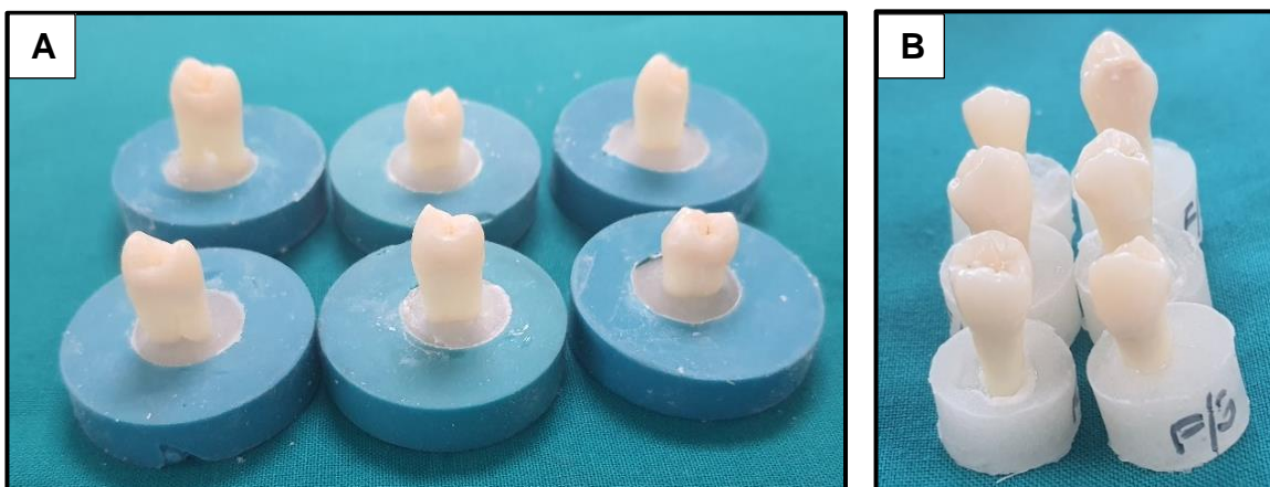
Figure 3-23: A) Silicone moulds used to embed the apices in acrylic resin, B) Apical foramina of the teeth sealed with acrylic resin, to prevent dye penetration.
