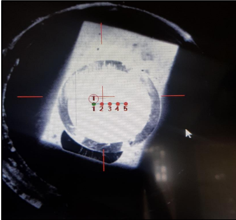
Figure 3-16: Five indentations in a straight line, no closer than 0.5mm to the adjacent indentation.
