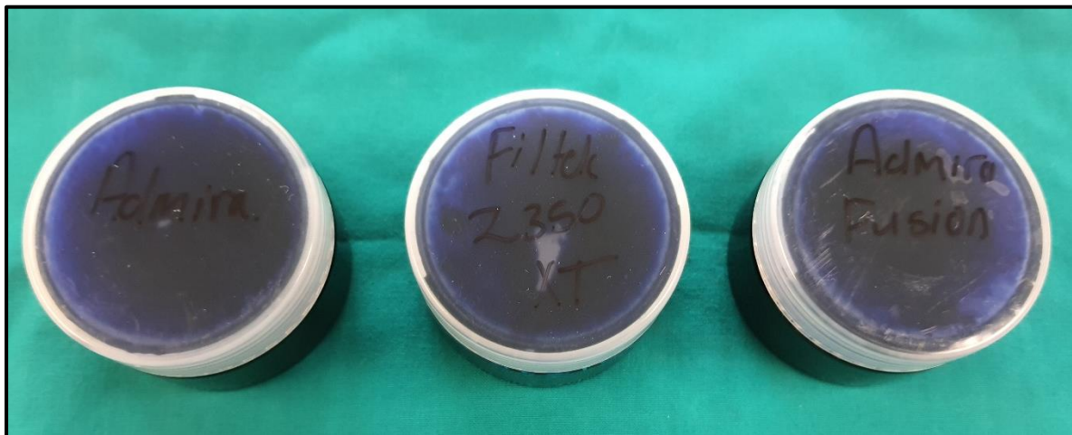
Figure 3-25: Samples immersed in 2% methylene blue dye solution for 48 hours.
