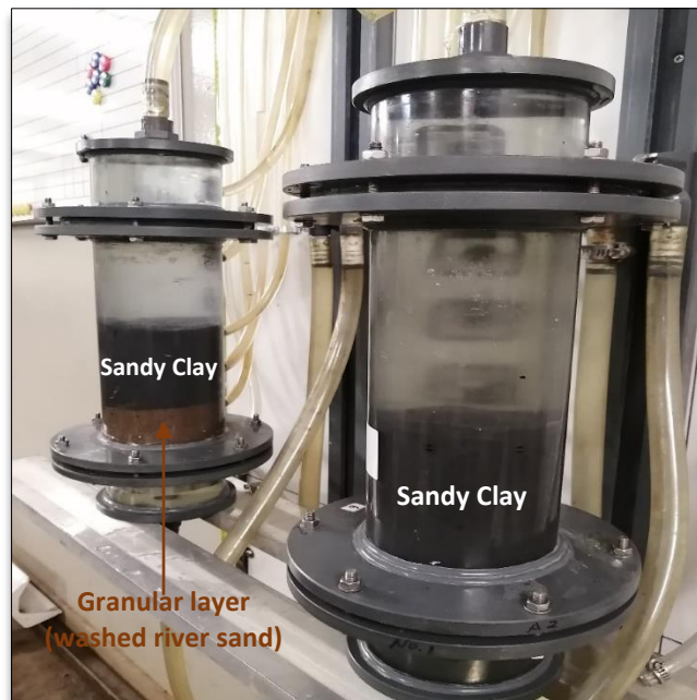
Figure 3: Permeameters during the filtration test. Test A is sandy clay and the granular layer. Test B is the sandy clay with no granular layer
